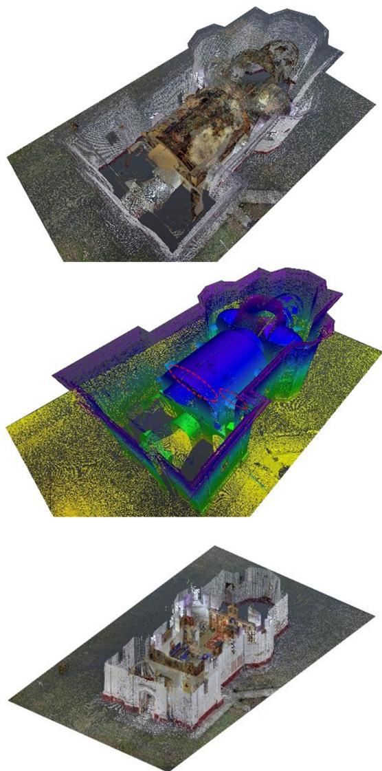
**Fig. 4.** 3D laser scanning of Bezdin church – cross-section
