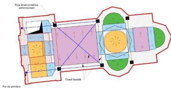
**Fig. 5.** System of flexible suspension cables
