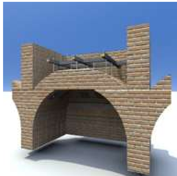
Fig. 18. Consolidation with beams of vaults [4]
