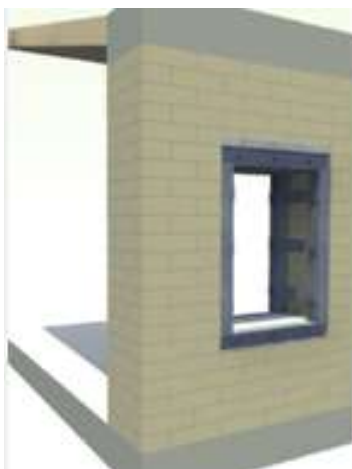
Fig. 16. Consolidation with steel profiles of openings [4]
