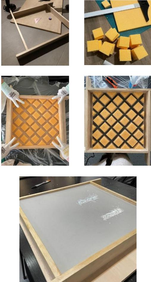
Fig. 3 Construction of the slab model
