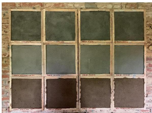
Fig. 5. Samples applied in situ, on the brick
