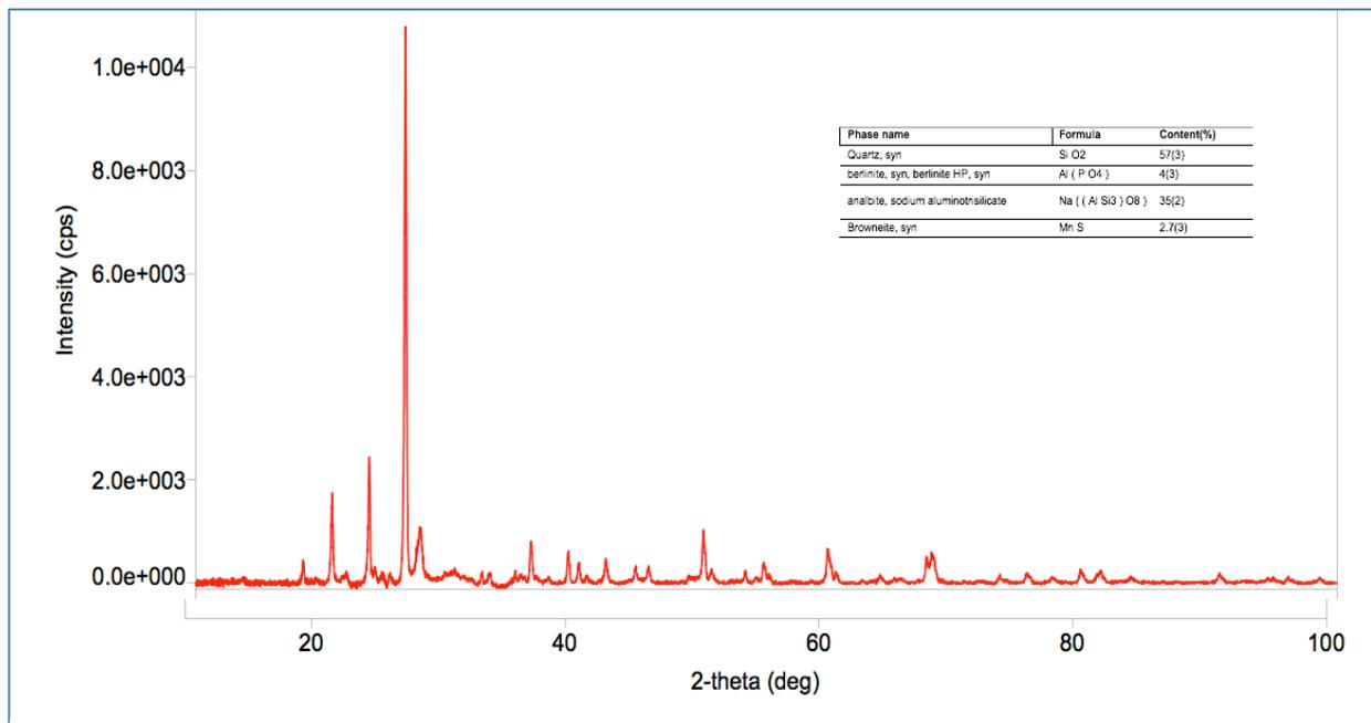
Fig. 6. XRD diagram of the original brick
