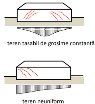
Fig. 2 Presentation of loads distribution in the foundation soil (from the course) [9]
