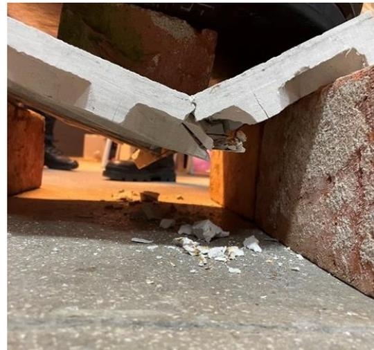
Fig. 5 Failure of the slab model
