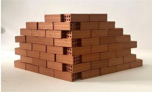
Fig. 1 Exploring different types of bonds for brick masonry structures – load-bearing solutions and aesthetic patterns
