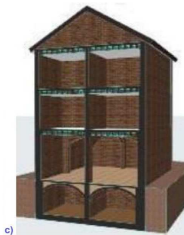
Fig. 8 Building class Type III
