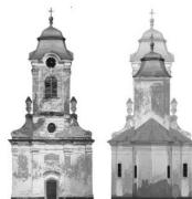
Fig. 3. 3D laser scanning of Bezdin church – façades
